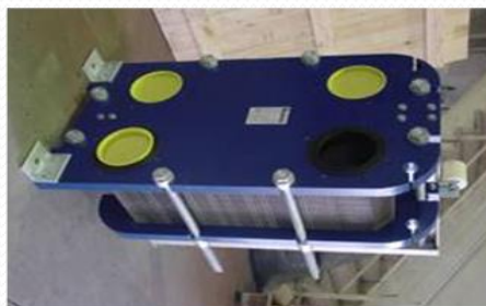
Plate Type Heat Exchanger
